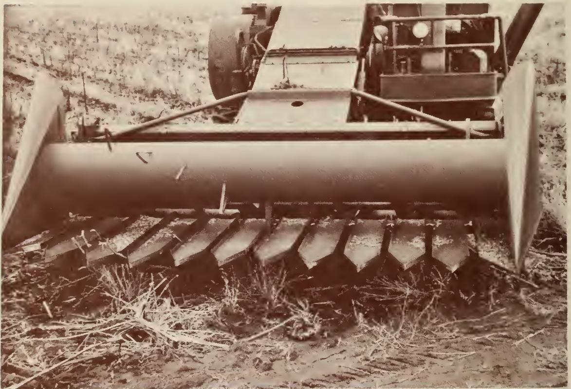
Figure 5 — Another type of harvesting attachment using a rotating drum to replace the conventional reel. This type of replacement is gaining popular acceptance. Other parts are similar to those shown in Figures 3 and 4.
