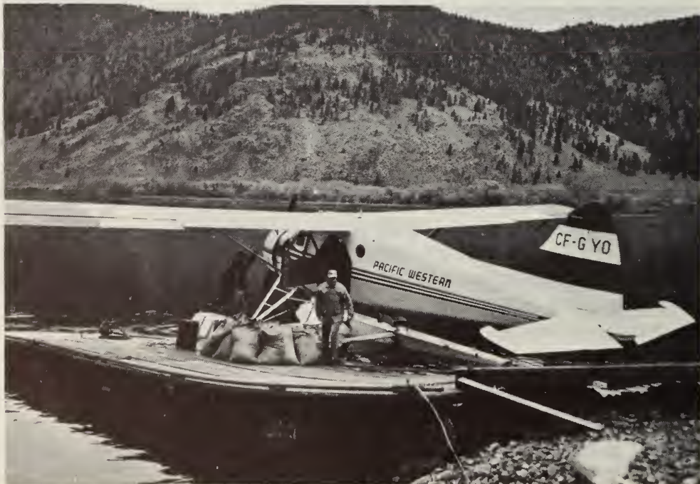
Figure 3.—A float plane rigged for seeding. This aircraft can carry 1,000 pounds of seed. Note the seeding spout protruding from the center of the fuselage.
