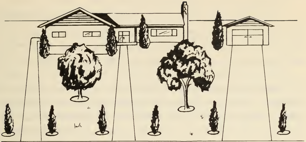
Fig. 2. Sketch illustrating a poorly designed approach planting. Lawn cut up into strips, and further encumbered by specimen trees and shrubs. Expense in maintaining this type of planning would be high, with extensive lawn edging in summer and snow removal in winter. Planting is monotonous and serves to accentuate the height of the buildings.
