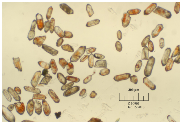
Figure 10901- 2 Transmitted light photomicrograph of zircon grains. Note high degree of alteration.
