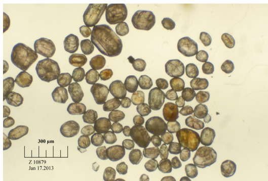
Figure 10879- 2: Transmitted light photomicrograph of zircon prior to mounting.
