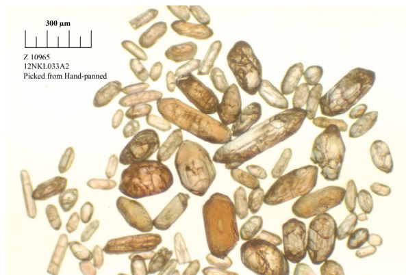
Figure 10965-2: Transmitted light photomicrograph of zircons recovered from the sample. Note variation in grain size and alteration.
