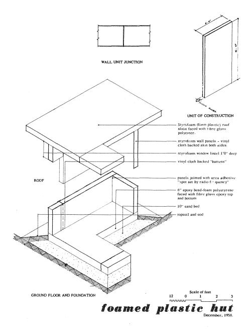
Figure 4-11. In the mid 1950s, CMHC and DBR built this demonstration house using plastic foams.
