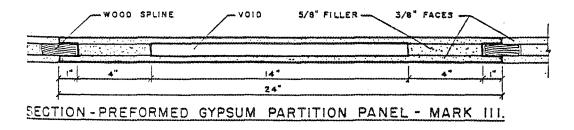
Figure 4-24. This drawing shows how the interior wall panels were constructed in the Mark III house.
