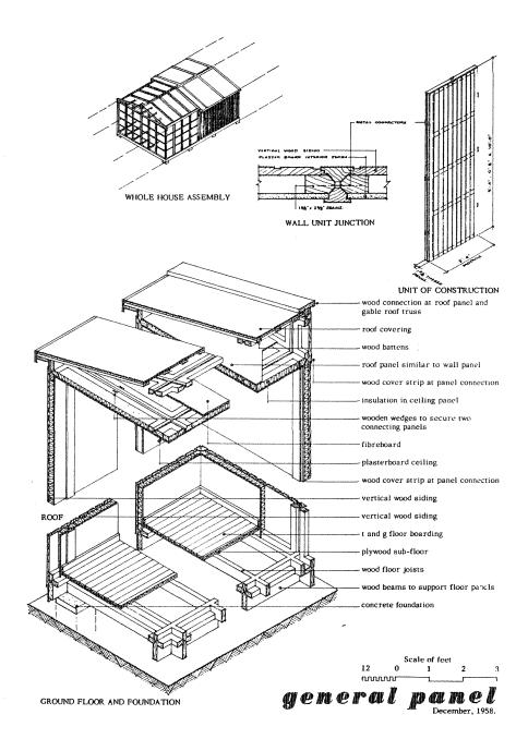
Figure 4-6. The General Panel Corporation, a United States firm, manufactured this prefabricated house in the late 1940s.
