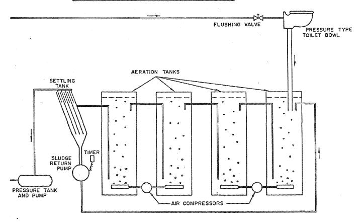
Figure 6-2. This drawing shows the configuration of the recirculating sewage system used in the Mark IV house.
