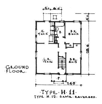
Figure 1-2. This was a typical floor plan for a small four bedroom house built by Wartime Housing Ltd.
