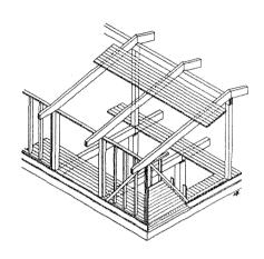
Figure 4-2. These two drawings show platform framing (left) and post and beam construction (right).
