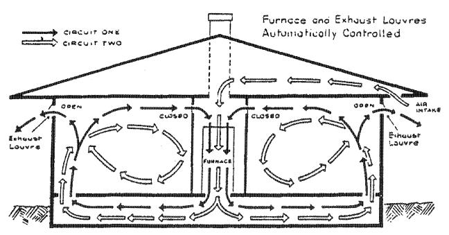
THIS DIAGRAMMATIC SKETCH shows the air flow in the heating and air-conditioning system of Experimental Project Mark III. White arrows indicate fresh air, black arrows, used air.
