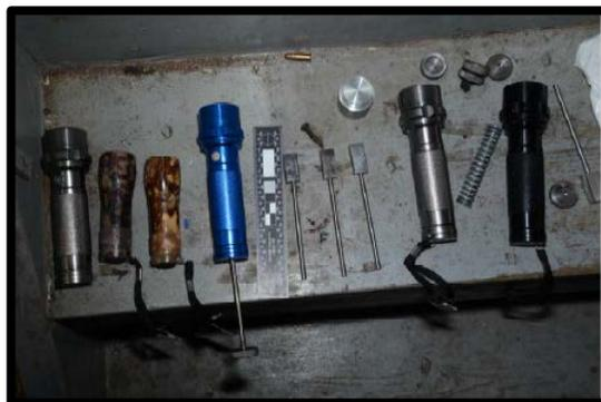
Flashlights in the process of being converted into firearms
