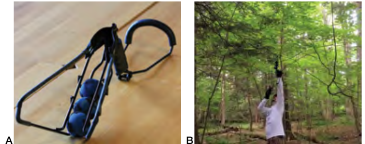
Figure 3. A) The Hyperdog™ ball launcher used in ball sampling with three Velcro®-covered racquet balls. B) Launching balls into the crown of hemlock (Photos: Jeffrey Fidgen).
