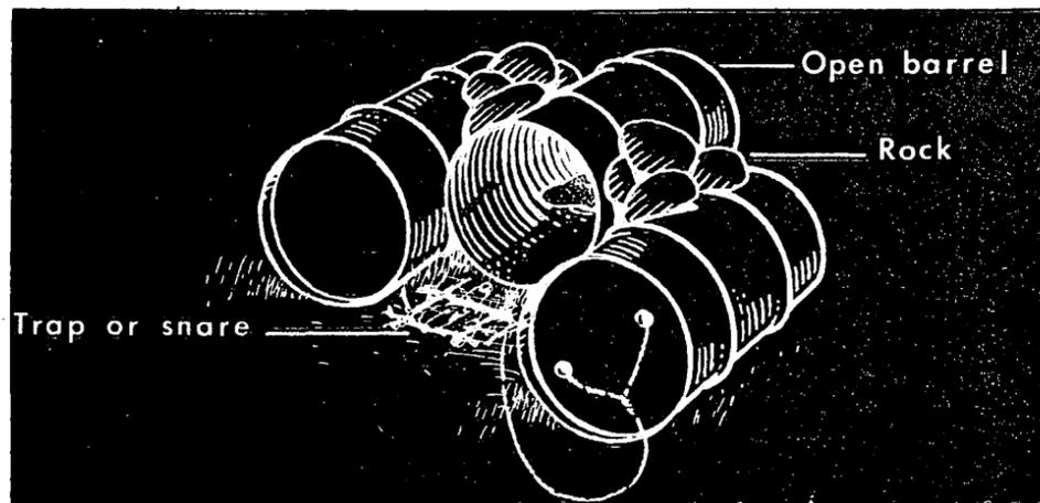
**Figure 2** A set built from three oil barrels, rocks, and sod. The centre barrel holds the bait and has one end open. The barrel on the right is partially filled with gravel and serves also as an anchor.
