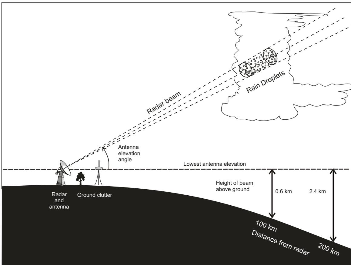
Radar scans this entire volume by raising and lowering the beam as the antenna rotates.
