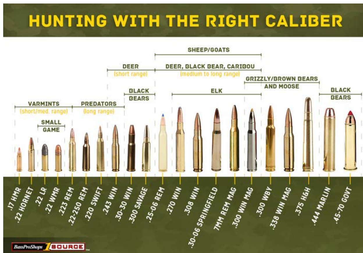
Figure 7. Illustration of Bullet Calibres
