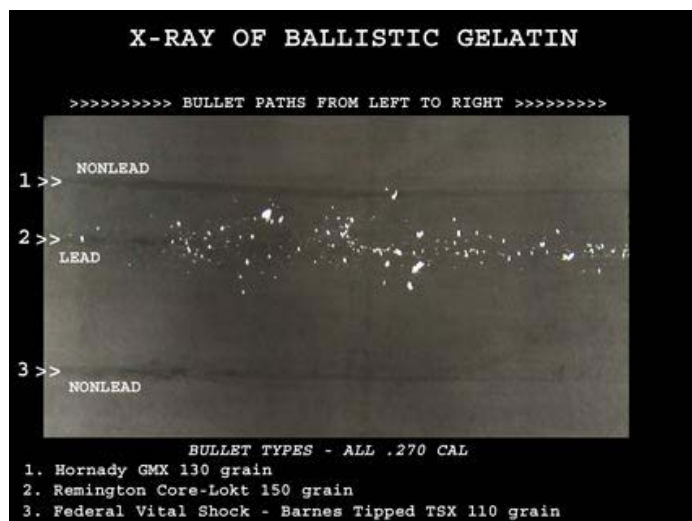
Figure 21. Non-Lead Hunting Bullets (100% Copper and 90% Copper) Comparable Ballistic Properties/Performance with Lead (X-Ray)
