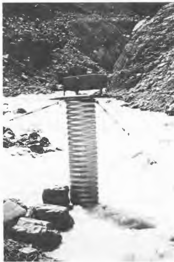
Figure 5. Steven's type A-35 water-level recorder, Peyto Creek
