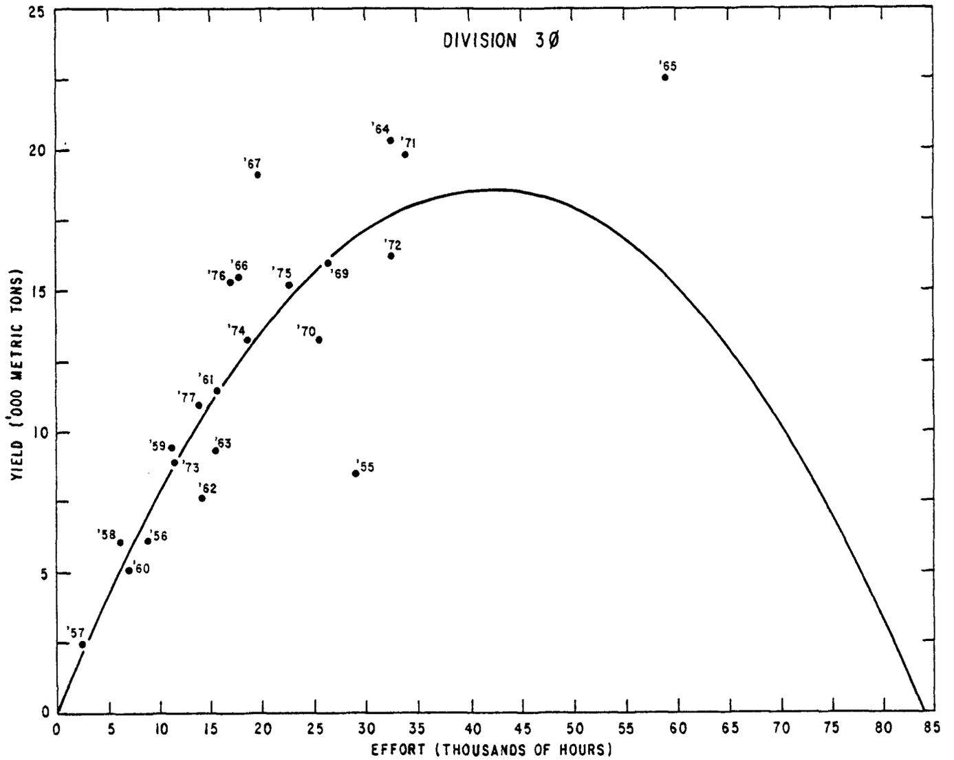
Fig. 3. Simple yield curve for Division 30 redfish derived from catch per unit effort for the standard hours fished from multiple linear regression.
