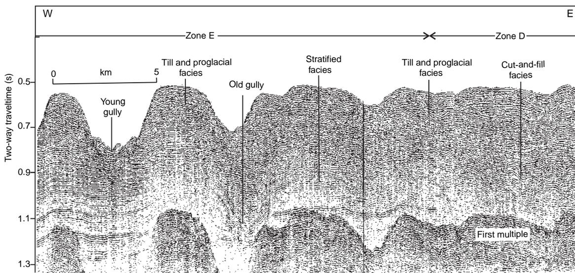
**Figure 8.** Seismic reflection profile along strike in 400 m water depth in zones D and E, showing gullies cutting till and proglacial facies overlying well stratified facies in zone E whereas in zone D, till and proglacial facies lack gullies and overlie cut-and-fill facies. One 40 cubic inch airgun source, cruise 90-002.
