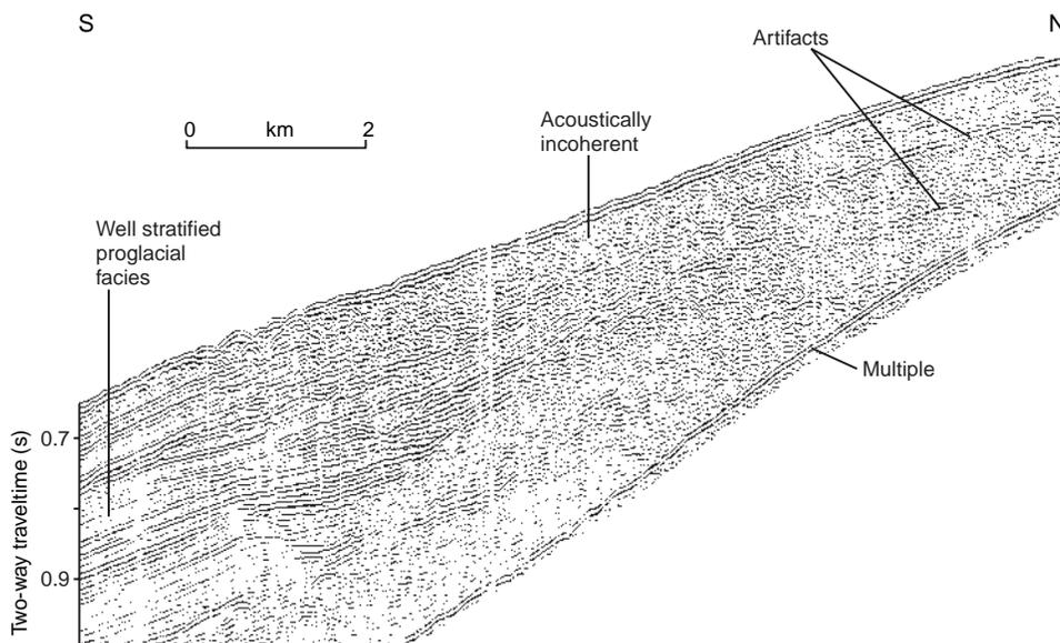
**Figure 6.** Seismic reflection profile down dip in zone D, showing incoherent acoustic facies corresponding to till passing downslope into well stratified acoustic facies, corresponding to proglacial plume fall-out deposits. One 40 cubic inch airgun source, cruise 90-002.
