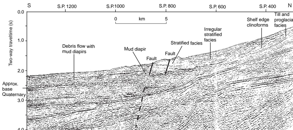
**Figure 9.** Industry multichannel seismic reflection profile down dip from the eastern end of zone A, showing late Cenozoic stratigraphy and facies. Petrocanada line 3416-82P courtesy Canada–Nova Scotia Offshore Petroleum Board.
