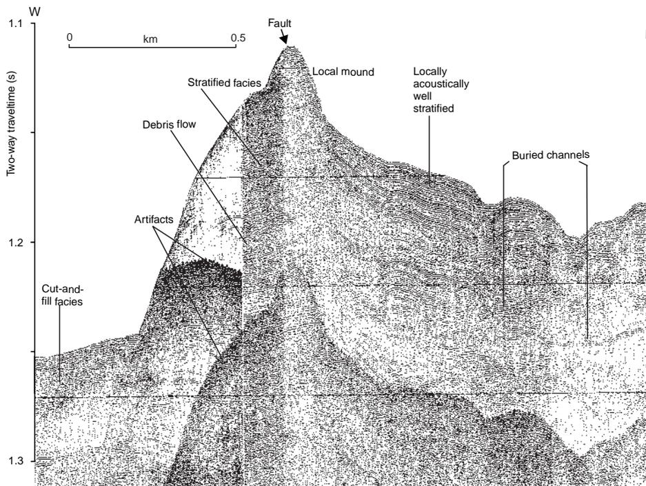
**Figure 4.** Huntec DTS™ sparker high-resolution seismic profile of part of the section in Figure 3 showing greater seismic resolution of facies, cruise 99-036.
