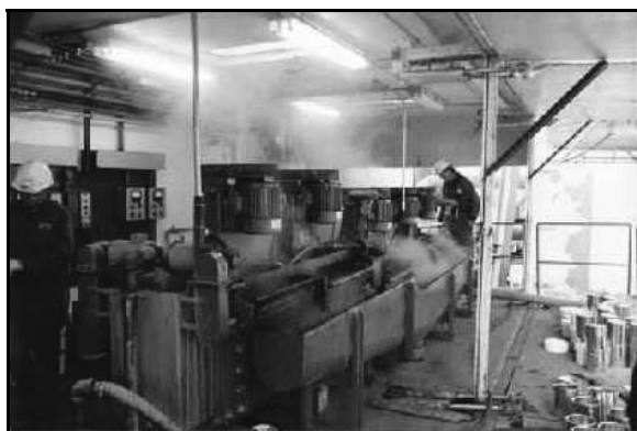
Bitumen recovery from tailings stream
