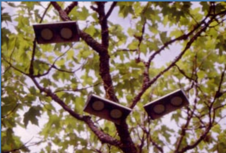
The CanOxy Plate™ passive ozone monitoring system (above) is being used by CFS and other agencies to measure the ozone trees are exposed to, right in the forest canopy (below).
