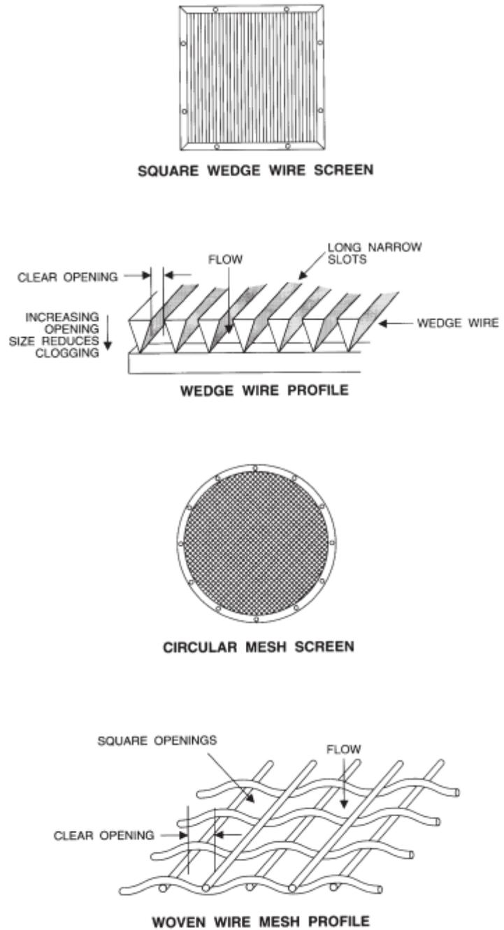
**Figure 5** Examples of Typical Installations of End-of-Pipe Screens
