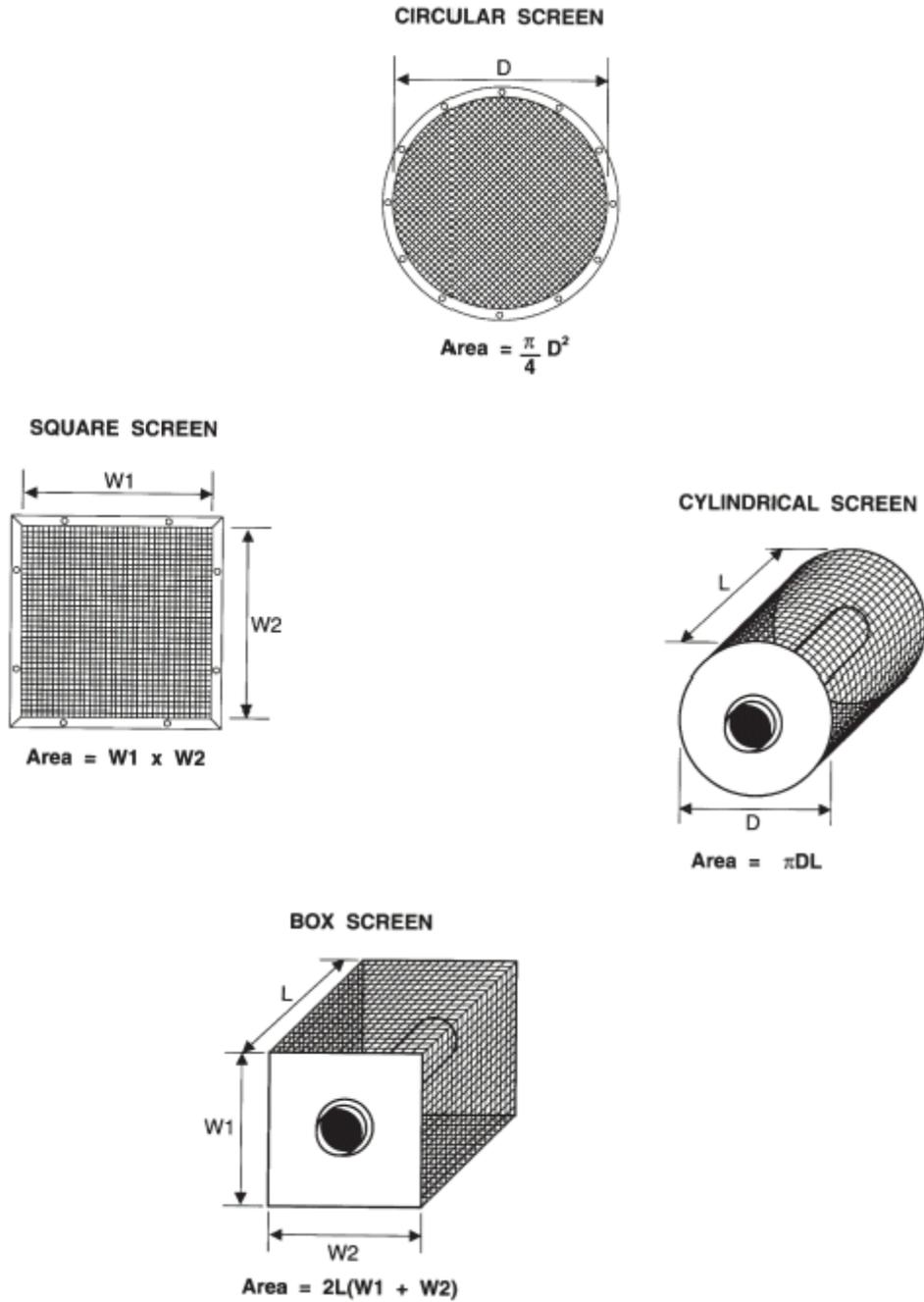
**Figure 3 Typical Applications and Features of End-of-Pipe Screens**
