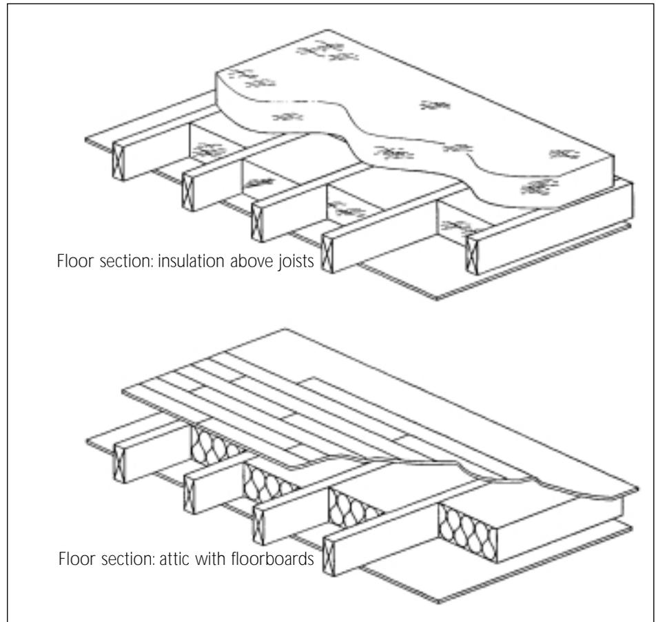
When walking in the attic in older houses, step only on the wooden joists that cover the floor. The joists are usually spaced every 16 inches. They are often hidden under a pile of insulation. If you step off the joists, you will probably put your foot through plaster or drywall
