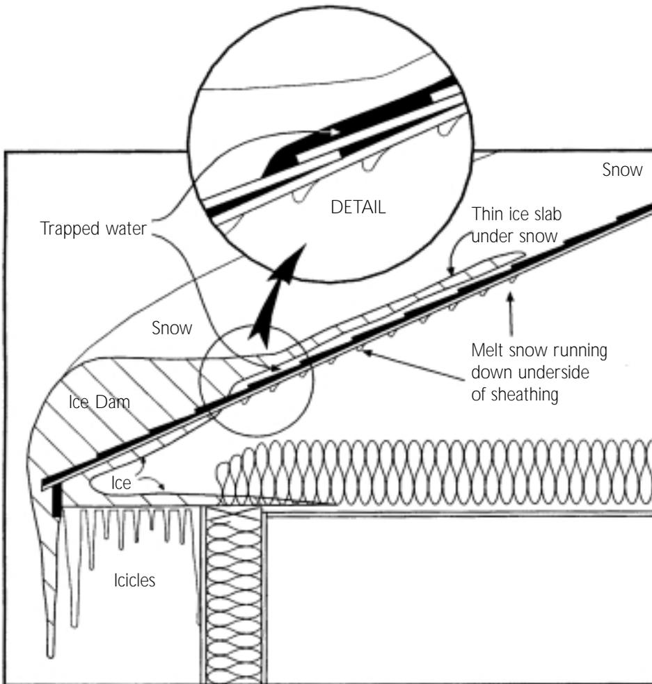
The basic relief for ice damming is to seal all attic air leaks and insulate thoroughly—the same as the attic condensation solution.
