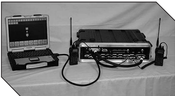
SyTech's portable Radio Inter Operability System (RIOS)
