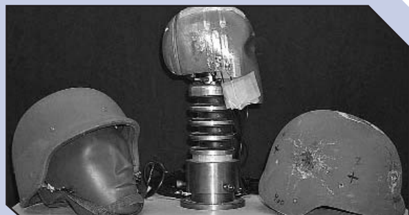
Ballistic testing equipment and helmets used in creating a new performance standard
