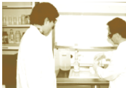
Michael Kwan (left) and Alix Gordon using acid to digest a tissue sample that will be analysed for mercury in the atomic absorption spectrometer. Photo: Nunavik Research Centre.
