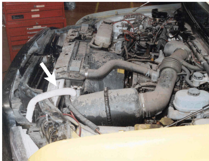
Photo 3. Discharge hose from the forward engine compartment
