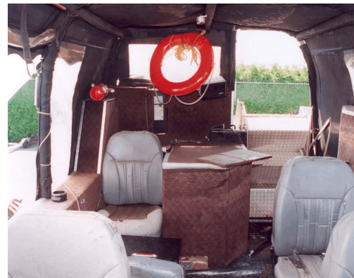
Photo 12. View from inside the vehicle of rear exit with boarding ramp in retracted position
