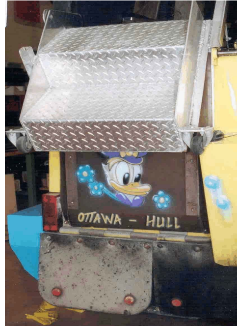
Photo 13. After boarding ramp in retracted position
