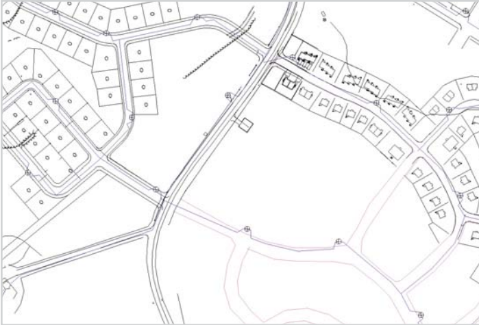
Figure 3 A GIS map of an expanding area of Mistissini. New residential lots are in the upper left of the map, and planned roads and the water and hydrant infrastructure are in the lower right.
