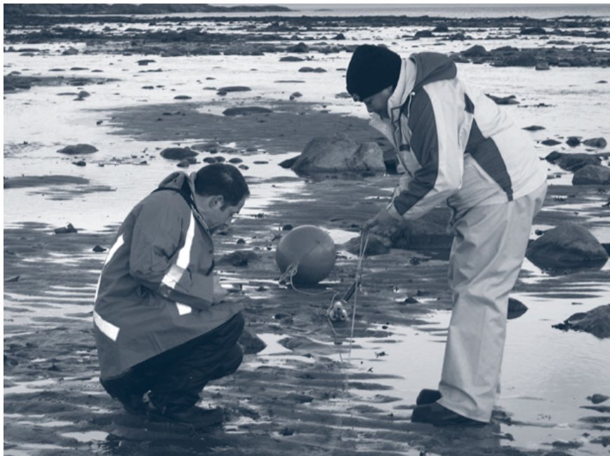
Figure 4 Students from Nunavut Arctic College preparing data logger to monitor temperature and pressure (depth) over a tidal cycle. A) enlargement of a data logger. Photo: T. Dick.
