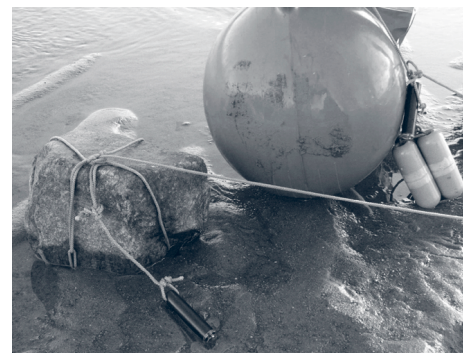
Figure 4 Students from Nunavut Arctic College preparing data logger to monitor temperature and pressure (depth) over a tidal cycle. A) enlargement of a data logger. Photo: T. Dick.
