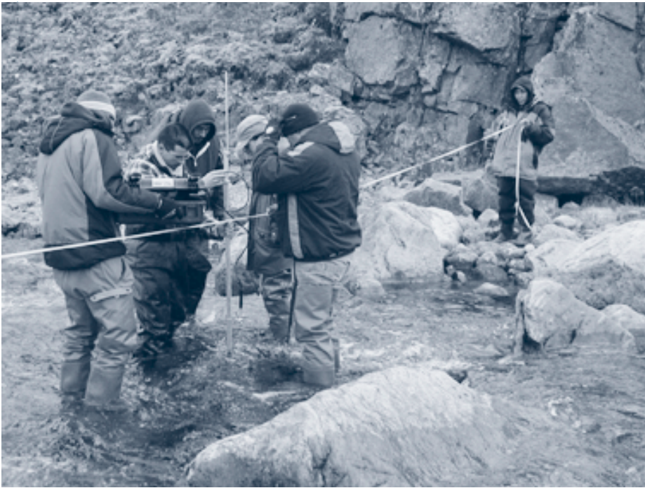
Figure 5 Students from Nunavut Arctic College using a portable acoustic flow meter to measure current across a stream bed so that total stream flow can be calculated. Photo: T. Dick.
