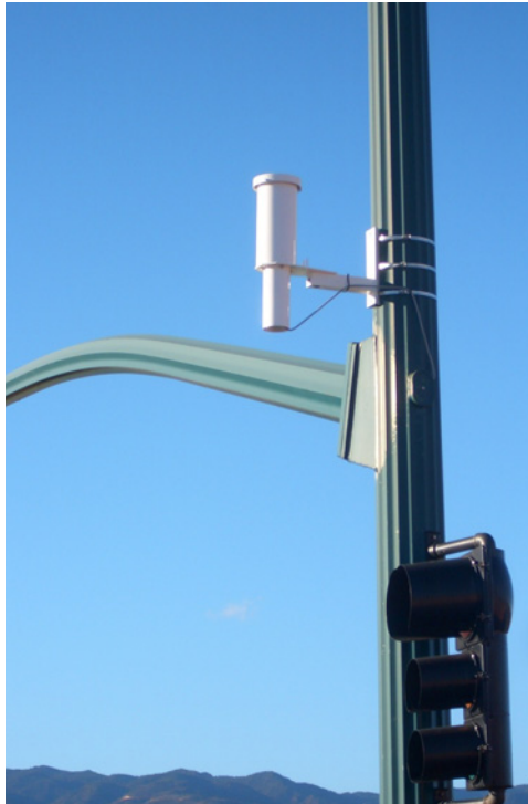
Mobile Detect equipment is deployed on a street lamp as part of a City of Colorado Springs pilot program to detect radiological materials in passing vehicles that could be used in weapons or other radiological contraband.
