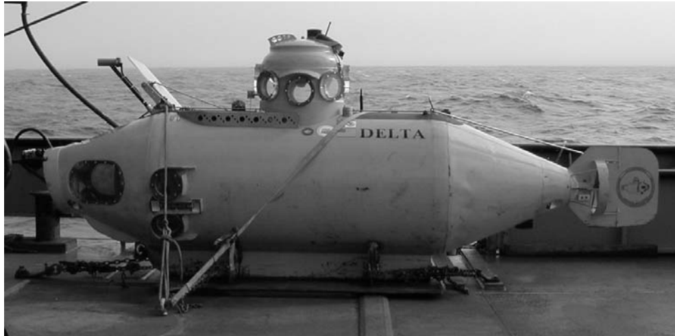
Figure 2. Two person submersible DELTA (Delta Oceanographics) on the deck of the CCGS John P. Tully.
