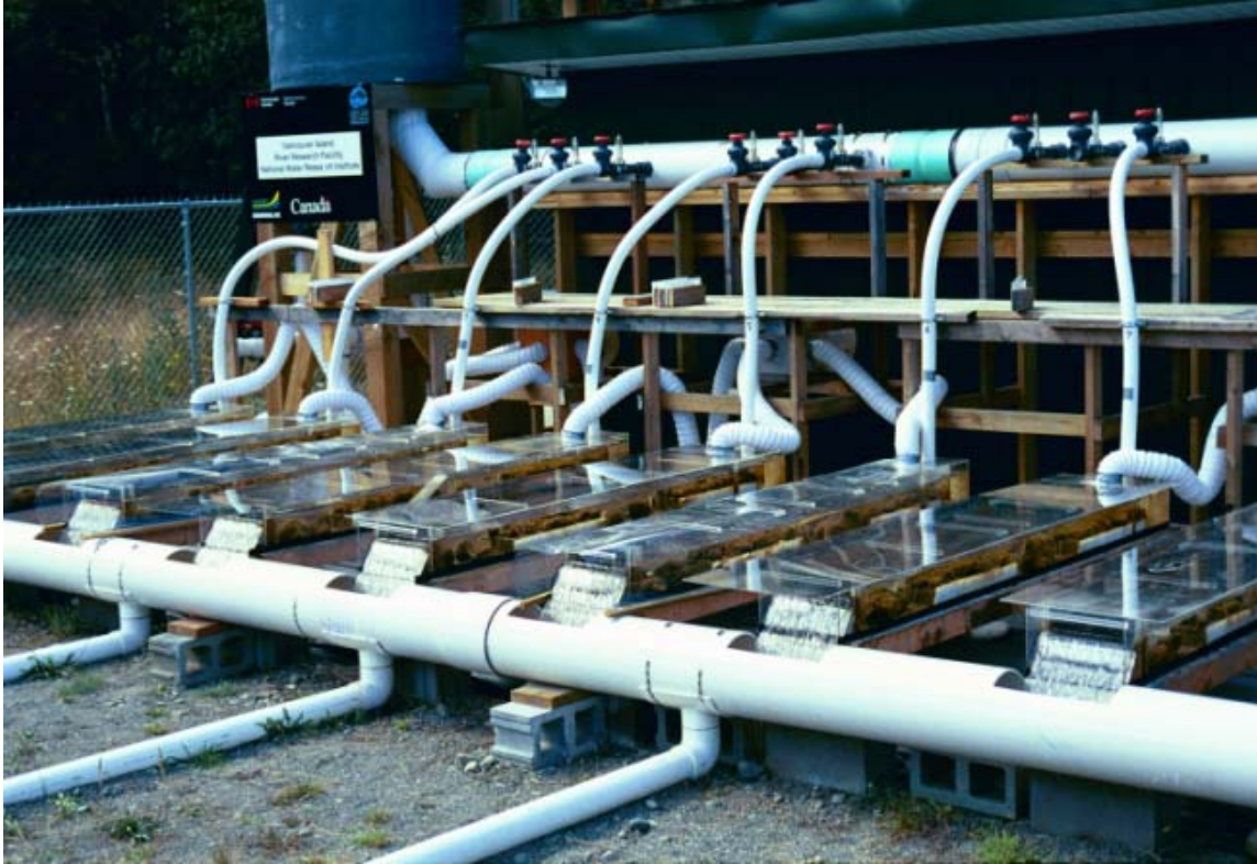
Figure 5. Mesocosm flumes at Little Qualicum exposing juvenile coho and the entire foodweb to sunlight with and without UVA and UVB radiation.
