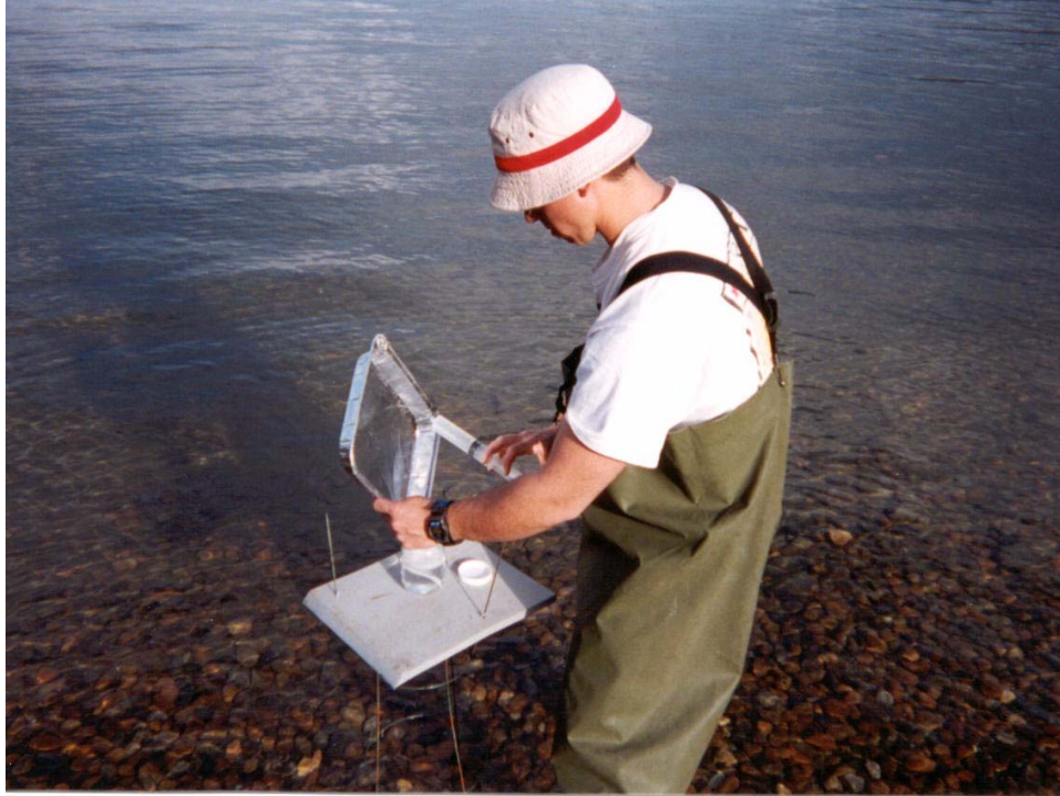
Figure 7. Insect water traps (aluminum trays filled with water and a drop of detergent) were used to sample insect input to the lake surface.
