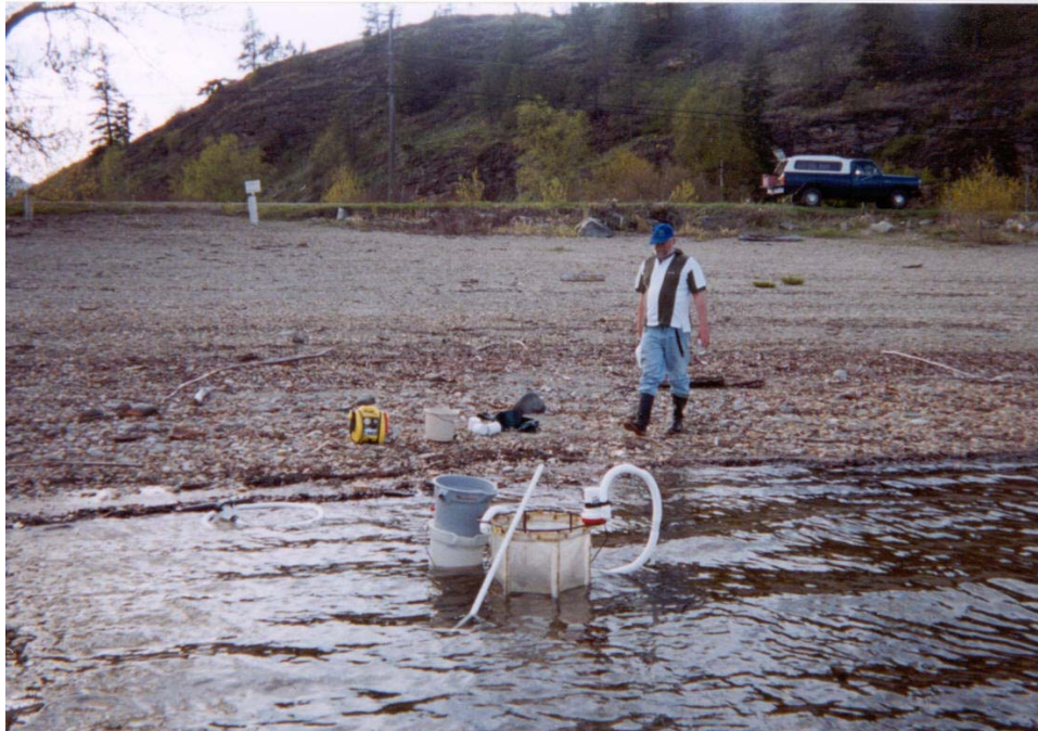
Figure 12. Benthic sampler using bilge pump to suck up invertebrates.
