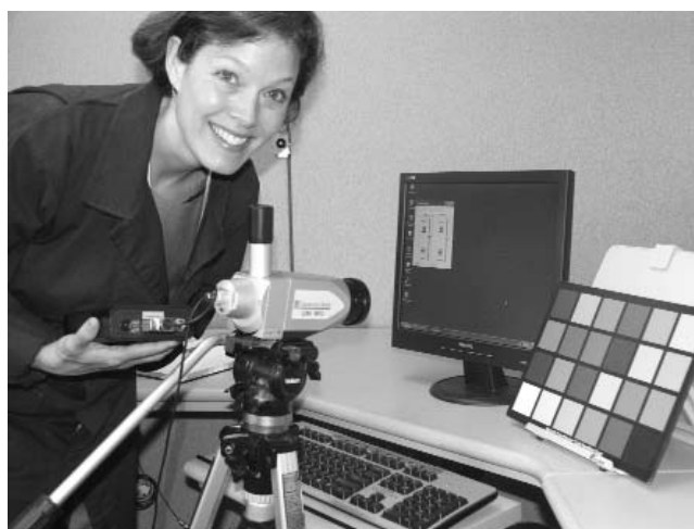
Dr. Jennifer Veitch uses a luminance meter to measure light exposure. Recent research suggests that people may benefit from more light each day than they usually receive.
