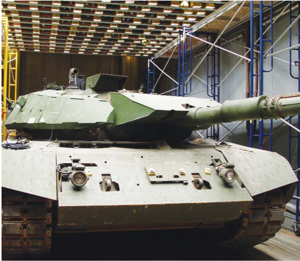
A Leopard tank bakes in a simulation of the midday Afghan sun.
