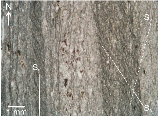
Figure 9. Photomicrograph showing a chevron cleavage pattern between S_2 (clockwise to S_0 ) and S_3 (counterclockwise to S_0 ) in the Jackson Lake Formation. The latter occurs only in the pelitic beds. Plane light. South of Jackson Lake.
