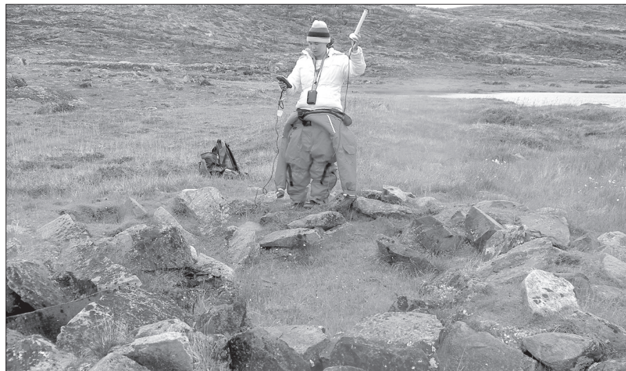
Kaviq Kaluraq of Baker Lake uses a DGPS (Differential Geographic Positioning System) to record the location of a Thule winter house at Tinnittuqtuq Point.
