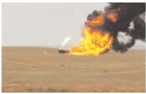
Figure 2. Initial Burning of Liquid Propane from Bottom of Tank
