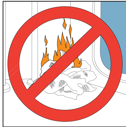
– Oil-soaked rags are often overlooked. They don't look as if they could start a fire. But in fact, they can burst into flames by spontaneous ignition – without any other source of heat! Always store oily rags in a non-flammable container.
