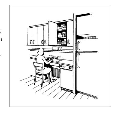
If you usually stand while using the sink, the sink should be at a height requiring minimal bending. If you wish to sit while using the sink, there should be knee space, and the sink and faucets should be positioned to require minimal stretching.
