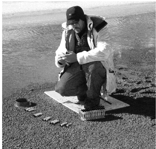
Figure 4b Surface fluxes of biogenic gases were made by collecting gases from collars inserted 10 cm into the soil. Soil temperature and water contents were measured at the time of sample collection. Samples were collected in evacuated vials and subsequent analyses were performed in the laboratory on a gas chromatograph.
