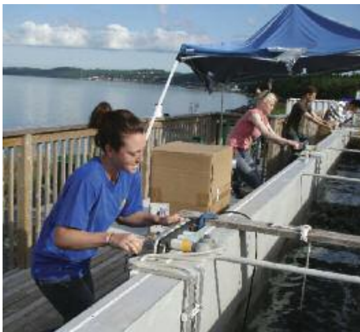
Figure 4. Summer students and COOGER staff recovering time-series samples from various depths within the wave tank to determine chemical dispersant effectiveness
