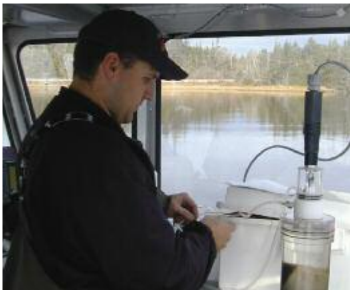
Figure 3. Brent Law of ERD operating the Microcosm Erosion Chamber to selectively erode flocs from the undisturbed surface of the core just acquired by the mini slo-corer.
