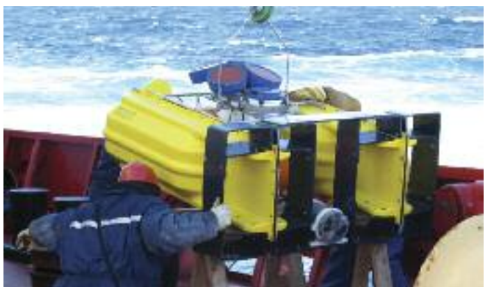
Deployment of an Acoustic Doppler Current Profiler to monitor ice drifts and ocean currents
