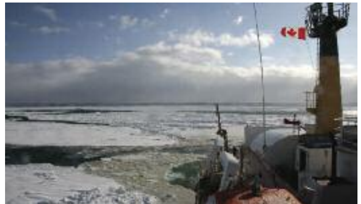
Figure 2. COOGER and Canadian Coast Guard collaborative field trial on combating oil spill on pack-ice conditions by delivering minerals and mixing using prop-wash from the ice-breaker, CCGS Martha L. Black
