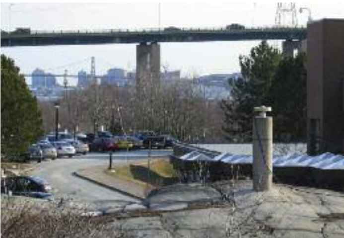
Figure 3. GPS antenna on pillar is set in bedrock above the front entrance to BIO, overlooking Halifax Harbour. This active control station operated by the Geodetic Survey Division of NRCan has been recording the position every second on a continuous basis since 2002. Weekly solutions are computed and used to estimate horizontal and vertical crustal motion.
