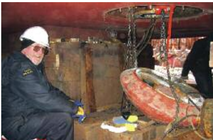
Replacing 12 Khz Transducer, Main Ram, CCGS Hudson , February 2007
