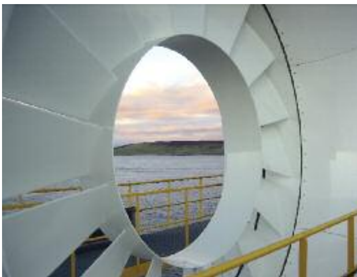
OpenHydro turbine prior to deployment in the UK – photo courtesy of Nova Scotia Power Incorporated
