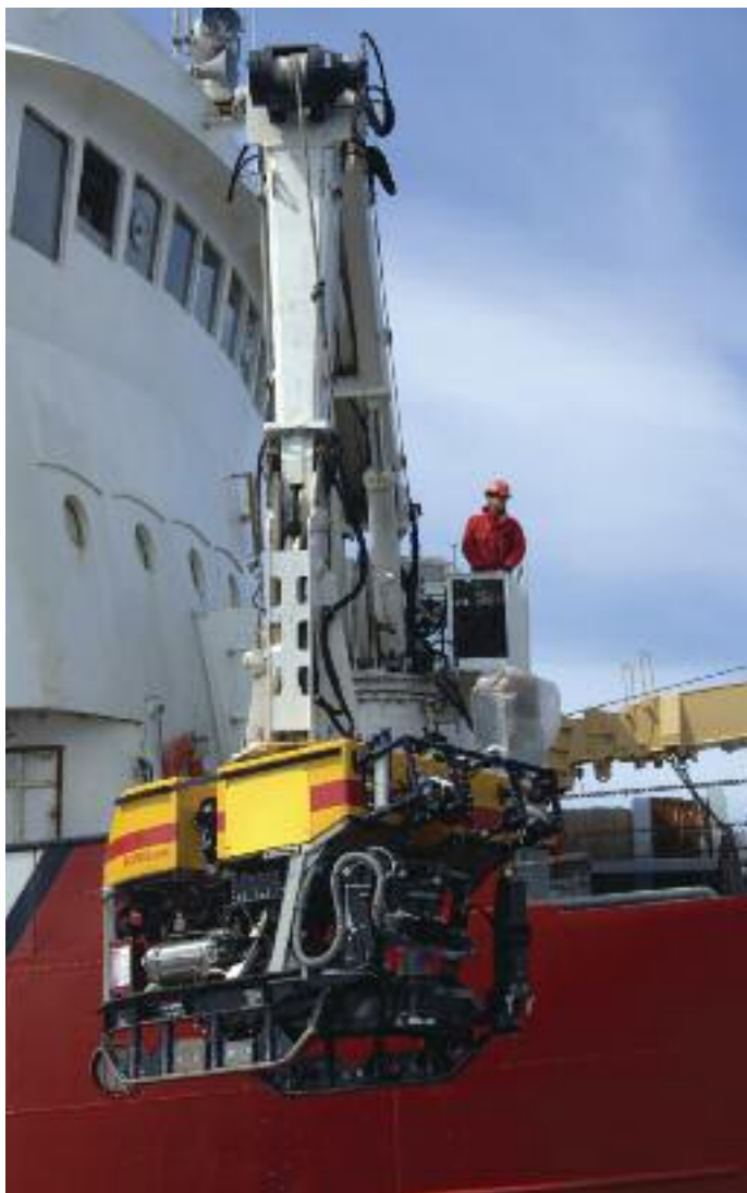
Figure 2. Deployment of ROPOS to explore the fauna in the deep waters of The Gully MPA
