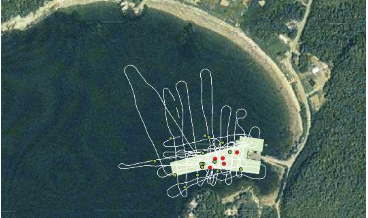
Figure 1. GIS presentation of Seeleys Cove: the aerial photograph shows the cove, beach, and wharf. The light green area is the area under consideration for dredging; the white line is the track of the survey vessel which measured water depth and sub-bottom sediment characteristics. The red dots are sediment core locations and the green dots are surficial grab-sample locations.
