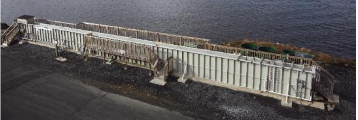
Figure 1. The wave tank at BIO is equipped with a computer-controlled wave maker to produce progressive non-breaking regular waves and breaking waves. It has been upgraded into a flow-through system to simulate movement of oil drops due to coexistence of waves and currents and to investigate dilution effects on toxicity of physically and chemically dispersed oil on pelagic and benthic species.
