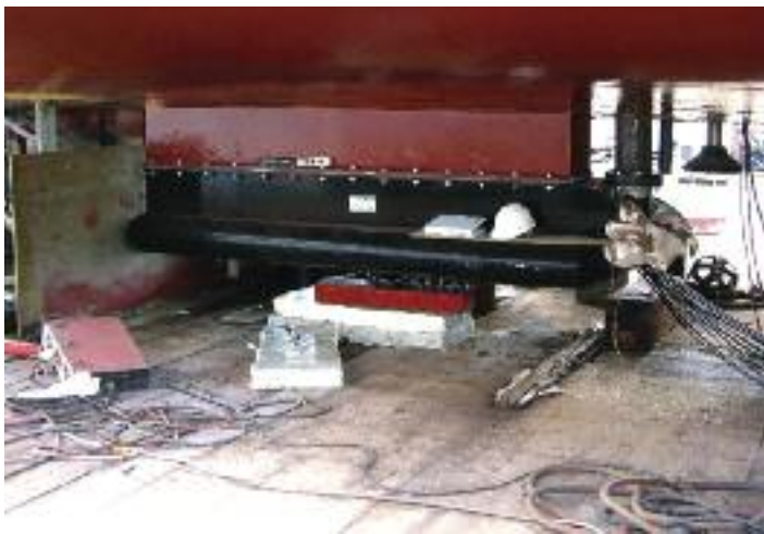
Installation of EM710 Transducer Array on the CCGS Matthew
