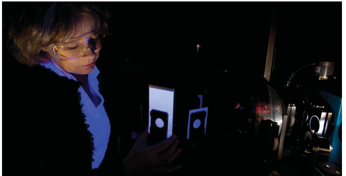
The "whiteness" of paper is a key component of its market value. NRC, which is recognized as the world authority in paper whiteness measurements, developed the reference instrument that establishes the absolute whiteness level for various types of paper.
