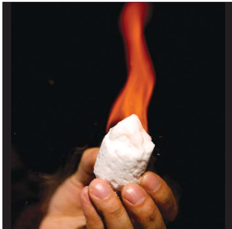
A gas hydrate is a crystalline solid consisting of water “cages” in which gaseous compounds, such as methane, are trapped one molecule at a time. At sufficiently high pressures, methane hydrates can remain “frozen” at temperatures above the melting point of ice, as shown in this “burning snowball”.
