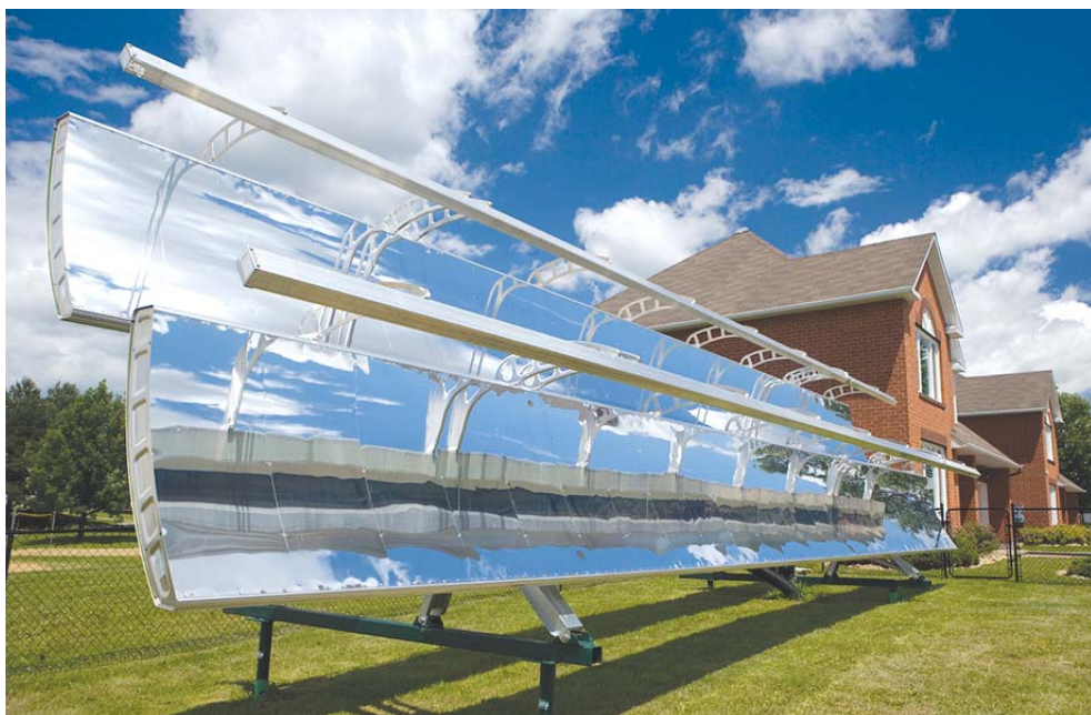
A solar concentrator system being evaluated at the CCHT test house.
