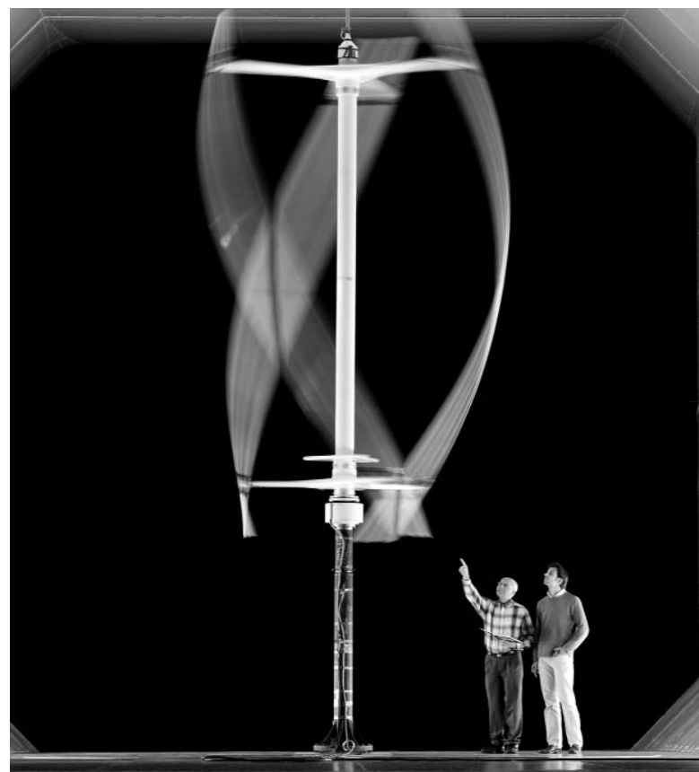
NRC research officer Paul Penna tests a vertical-axis wind turbine with Dr. Tamás Bertényi of Quiet Revolution.
