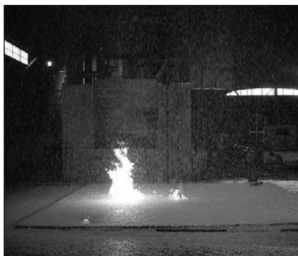
CAF extinguishes a free-flowing heptane spill fire in 38 seconds.
