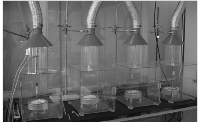
NRC-IRC's facility is used to test the propensity of different types of cigarettes to ignite materials.
