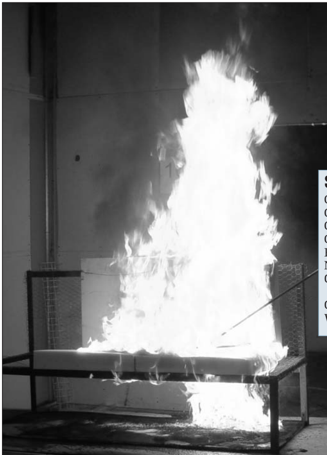
Mock-up sofa undergoing fire test to determine its burning characteristics
