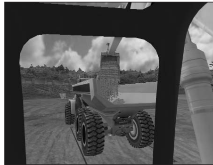
Personal simulator for heavy equipment training features realistic “virtual digging.”
