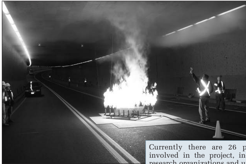
Full-scale fire test conducted by NRC-IRC researchers in a Montreal road tunnel
