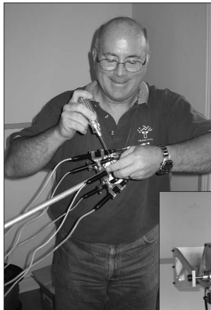
NRC-IRC researcher, James Reardon, installs sensors (above) on the robot arm (right).
