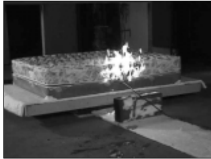
Using the FTIR technique to analyze smoke from a burning mattress
