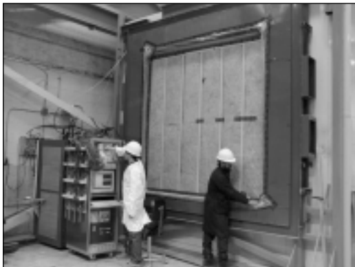
IRC researchers prepare full-scale wall specimen for a drying experiment in the Envelope Environmental Exposure Facility (EEEF)
