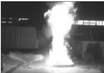
Gasoline fire at time of CAF activation
