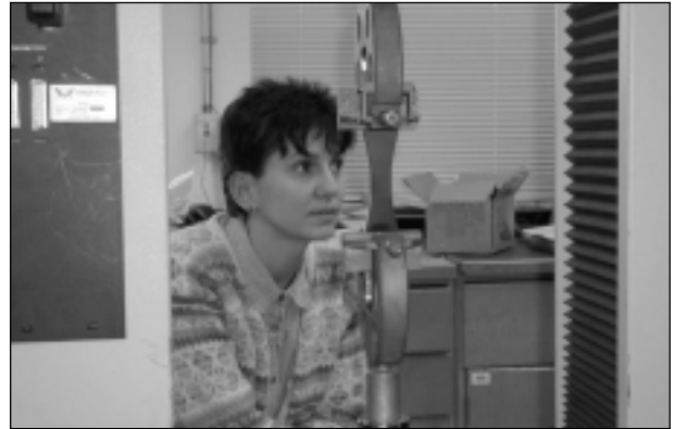
IRC technical officer, Lyne Daigle, tests high-density polyethylene pipe samples to determine their tensile performance.
