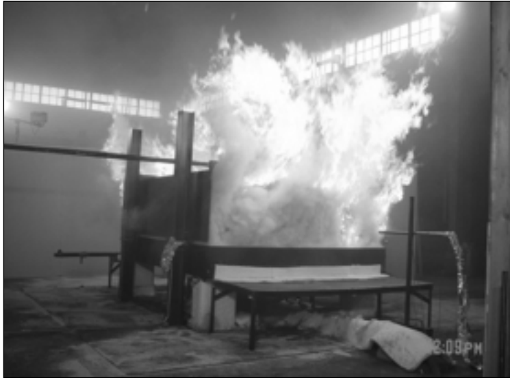
Mock-up used to test effectiveness of water mist in extinguishing large-scale cooking oil fires.
