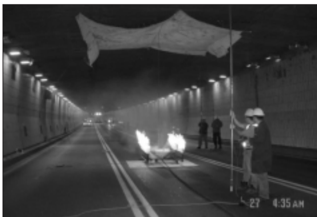
Researchers use propane burner to simulate a fire in Montreal's Louis-Hippolyte-La Fontaine Tunnel.
