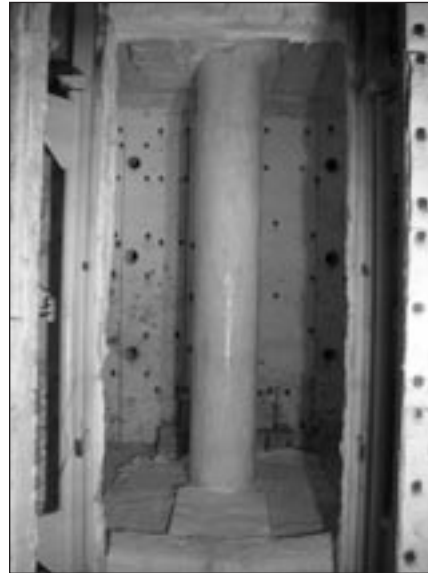
Typical circular, insulated FRP-strengthened concrete column before and after fire testing
