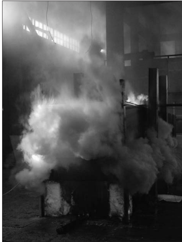
The MistShield water-mist system developed by IRC and CAFS Unit is able to effectively extinguish large-scale cooking oil fires.
