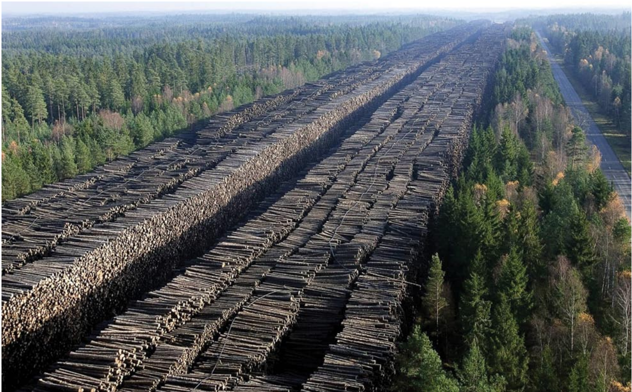
Figure 2. Approximately 1 million m 3 of Norway spruce sawlogs are being stored up to four years under sprinklers at an abandoned airstrip near Byholma, Sweden, by Vida Oy. The storage piles are about 13 m high, and the area used for log storage is about 60 m wide and 2.3 km in length.
