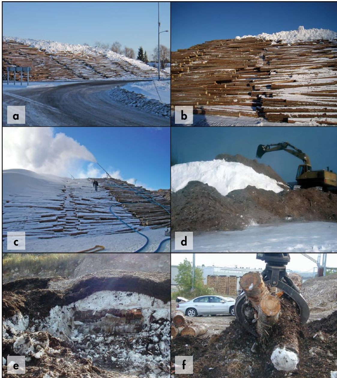
Figure 1. (a and b) In late winter, frozen logs are decked on level, frozen ground at Myllykowski Paper Oy near Simpele, Finland. Note that the sides of deck are angled to prevent sloughing of snowpack, the logs are tightly packed, and gaps between rows on the top layer are covered to prevent development of sinkholes. Photos: R. Whitehead. (c) A 50,000-m 3 cache is being covered with a 0.75-m-thick layer of artificial snow at UPM-Kymmene Oy near Kaipola, Finland. Photo: R. Whitehead. (d) A 0.7-m layer of spruce bark is being added to insulate a snow cache at the Kruger Sawmill in Parent, QC. Note that the insulation must protect from both rain and solar heating. Photo: J. Nader. (e and f) At end of the summer, when insulation is removed to allow snow to melt and to recover logs for processing at Produits Forestiers Bellerive Ka'n'enda Inc. near Mont-Laurier, QC, the snowpack is still intact and logs are still frozen and fresh. Photos: J. Nader.
