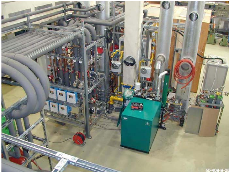
Figure III-1.4 : Equipment under test and hydraulic rack
