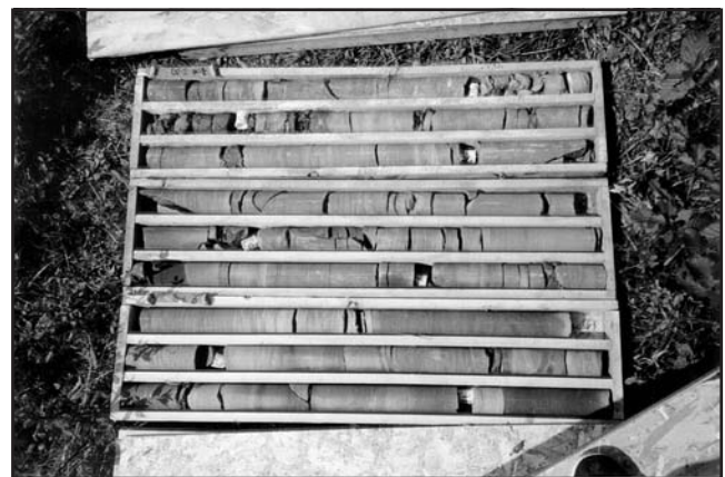
Figure 3. Core samples from diamond-drill hole, Légerville, New Brunswick. Core diameter 6.4 cm (2.5 inches).
